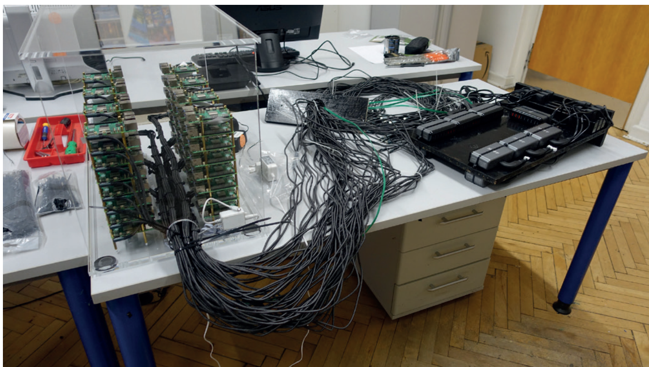
The Raspberry cluster is powered by 64 separate cables connected to 13 power supplies, each with 5 outputs.
